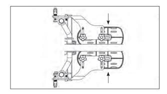
**Toe-in/Toe-out**-Loosen knobs underneath foot plates, slide foot plates into position. Tighten knobs securely.
