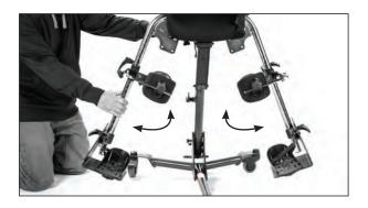
Twist until the knob is vertical and locks into position. The gas spring is now locked from unintended movement.
