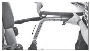
8. Insert tray tube into the tray bracket at desired height.
