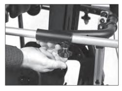
Move the tray surface to the desired angle and re-tighten both lever clamps securely.
