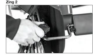
To adjust the fore/aft positioning on the hip supports, loosen the thumb knobs, adjust to desired position and tighten securely. **Zing 1 and Zing 2**
