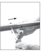
13. Use a hex wrench and 13mm wrench and remove nut and washer. Place into desired position. Use a hex wrench and 13mm wrench and tighten securely. Place black protective cap onto nut.
