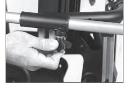
**Swing-Away Shadow Tray Adjustment** To swing-away tray, loosen one knob and swing tray away.
