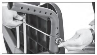
5. Remove black protective cap from the nut. Use a hex wrench and 13mm wrench and remove nut and washer.
