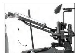
Swing-Away & Shadow Tray Adjustment To adjust the tray height, loosen both knobs on the back of the unit and set to desired position. Tighten knobs securely.
