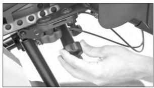
Adjusting to a shorter setting: Adjust the following arm (back angle) first by depressing the spring button and moving no more than two holes at a time. Then adjust the seat tube (seat depth) one hole at a time. Continue this sequence until you achieve the desired setting and the colors on the seat tube and following arm match.
