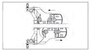
**Abduction**-Loosen ratchet handles to spread apart foot plates, tighten securely. Loosen knobs under foot plates and slide foot plates apart. Tighten knobs securely.
