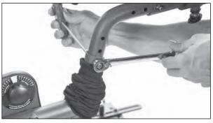
2. Use a hex wrench and 13mm wrench and remove nut and washer.
