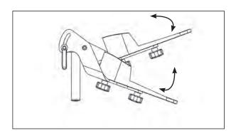
**Forward/Aft**-Loosen knobs underneath foot plates, slide foot plates into position. Tighten knobs securely.
