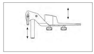
**Abduction**-Loosen knobs to slide foot plates together. Tighten knobs securely.
