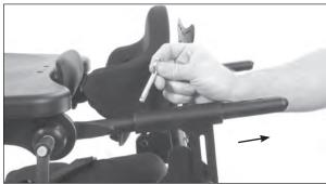
To adjust the height of the tray, loosen both ratchet handles on the side of the unit and lift the tray to the user's desired height, tighten securely.
