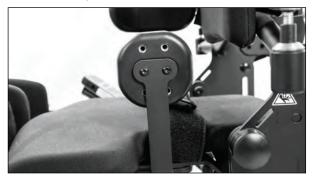
The lateral supports have a number of attachment holes on the back of the pad allowing for additional positions vertically and horizontally. The pads can also be bolted on at a straight, 90°, 180°, or 270° position.
