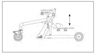
**Adduction**-Loosen knobs to slide foot plates together. Tighten knobs securely.
