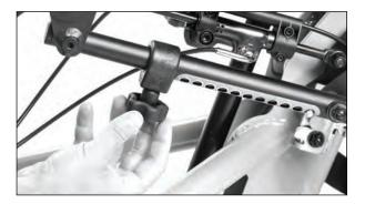
Adjusting to a longer setting: Adjust the seat tube (seat depth) first by depressing the spring button and moving only one hole at a time. Then adjust the following arm (back angle) no more than two holes at a time. Continue this sequence until you achieve the desired setting and the colors on the seat tube and following arm match.
