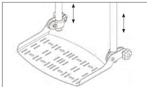
Multi-Adjustable Foot Plates Height-Loosen the ratchet handles connecting the foot bracket to vertical leg tubes to adjust foot plate height.
