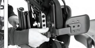
To adjust the lateral support height, loosen knob, adjust to desired position. Tighten securely.
